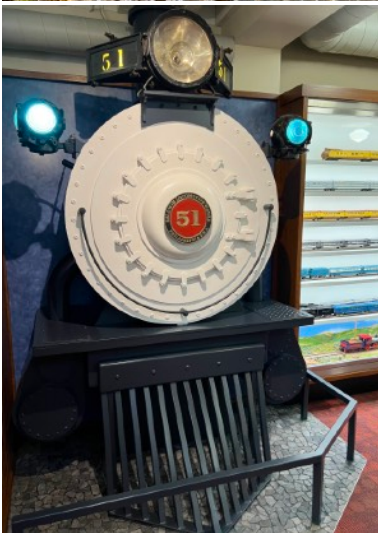
Full-size boiler front with original headlight and marker lights.
